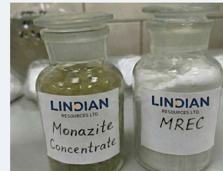
Monazite concentrate from Kangankunde and the resulting MREC product produced at the SARECO facility
